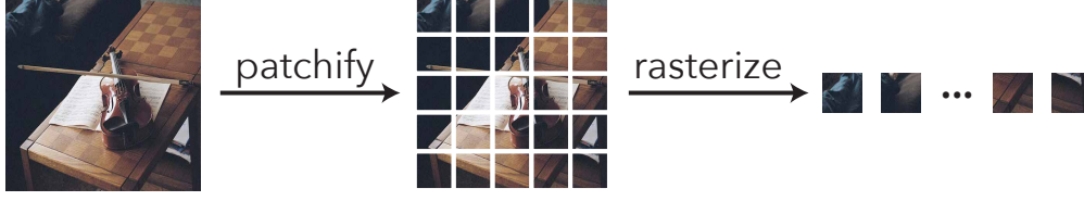
Figure 7.5: An example of an image turned into 5 \times 5 square patches, which are placed in raster order. Each patch is of the same size, and the grid of patches is of shape (N_H, N_W) = (5, 5) . The grid of patches is then unrolled into a sequence of length 5 \times 5 = 25 in raster order.
